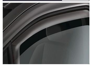
Wind deflectors are ideal if you like to drive with the windows open. They are custom designed to match the aerodynamic contours of your vehicle and work by diverting air flow to ensure that you and your passengers are not troubled by excessive wind movement and noise.
